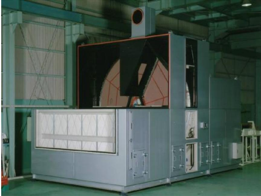
The rotor-concentrator / thermal oxidiser is the most cost-effective technology for treating large volumes with low VOC concentrations. The real savings come from reduced operating costs.
