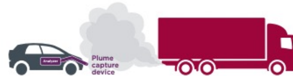
Figure 3a: Schematic setup of a plume chaser installed in vehicle measuring the exhaust emissions from the truck in front
