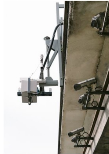
Figure 3-2: The EDAR unit mounted on a gantry
