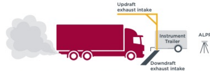
Figure 3b: Schematic setup of a stationary air sampling system.
