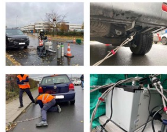
Figure 4. Remote sensing emissions testing and particle number inspections of vehicles at the BRU0019 site on Rue du Lieutenant Lotin.
