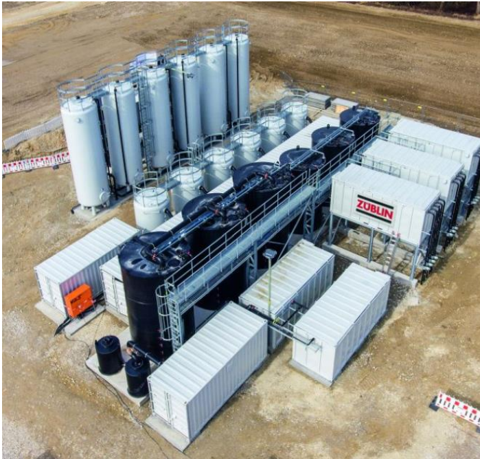
Former refinery – hydraulic barrier, 200 m 3 /h
