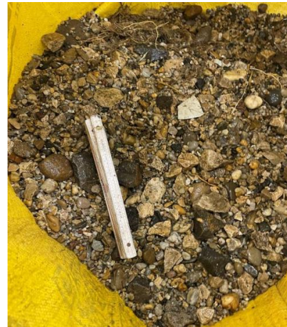
Gravel (> 2,5 mm), 11.0% wt. Sand (< 2,5 mm): 63.8% wt. Fines (< 0,63 µm): 24.5% wt.
