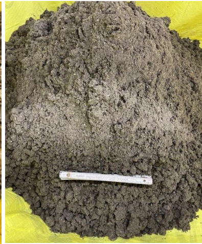
Gravel (> 2,5 mm), 11.0% wt. Sand (< 2,5 mm): 63.8% wt. Fines (< 0,63 µm): 24.5% wt.
