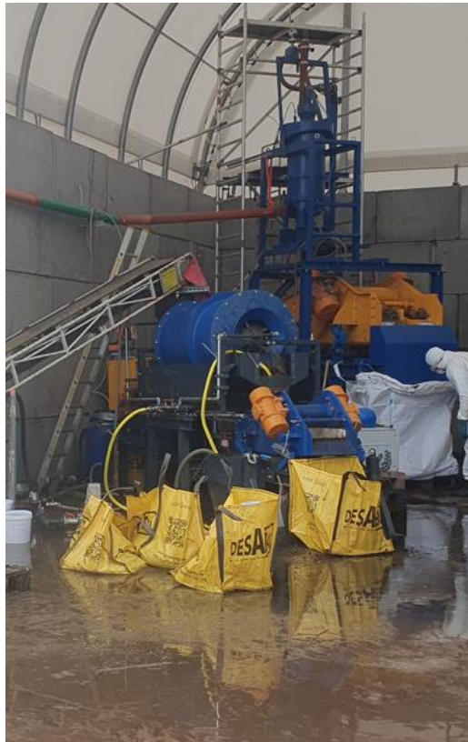
Soil washing plant, multi-stage, technical scale
